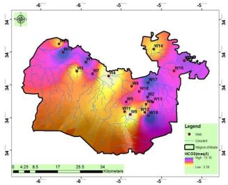
**Figure 6:** Spatial distribution of bicarbonate ions (HCO<sub>3</sub>) of water samples from the study areas in Sidi Slimane, Morocco.
