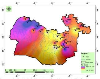
**Figure 4:** Spatial disbisution of sodium ions (Na<sup>+</sup>) of water samples from the study areas in Sidi Slimane, Morocco.
