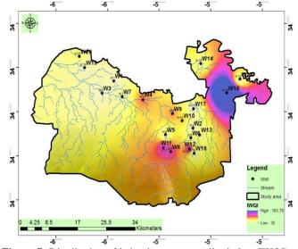
**Figure 7:** Distribution of irrigation water quality index (IWQI) of water samples from the study areas in Sidi Slimane, Morocco.
