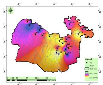
**Figure 3:** Spatial distribution of sodium adsorption ratio (SAR) of water samples from the study areas in Sidi Slimane, Morocco.
