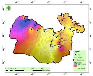
**Figure 2:** Spatial distribution of electrical conductivity of water samples from the study areas in Sidi Slimane, Morocco.
