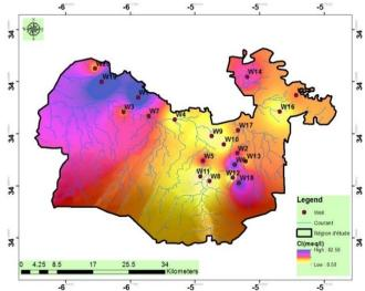
**Figure 5:** Spatial distribution of chloride ions (Cl<sup>-</sup>) of water samples from the study areas in Sidi Slimane, Morocco.
