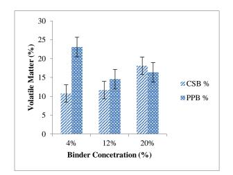
Figure 2: Effect of binder type on volatile matter of fuel briquette.
