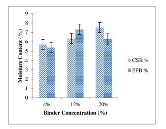
Figure 1: Effect of binder type on moisture content of fuel briquette.
