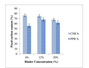
Figure 3: Effect of binder type on fixed carbon content of fuel briquette.
