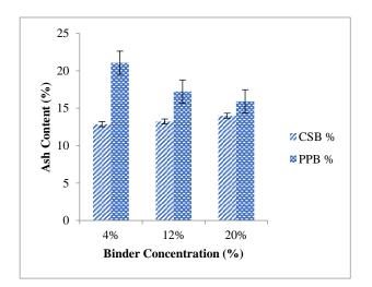
Figure 4: Effect of binder type on ash content of fuel briquette.
