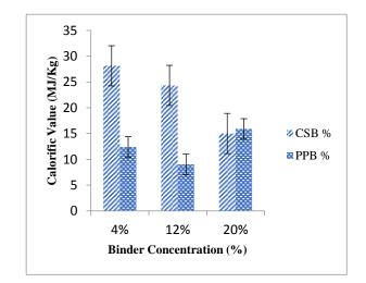
**Figure 5:** Effect of binder type on calorific value of fuel briquette.
