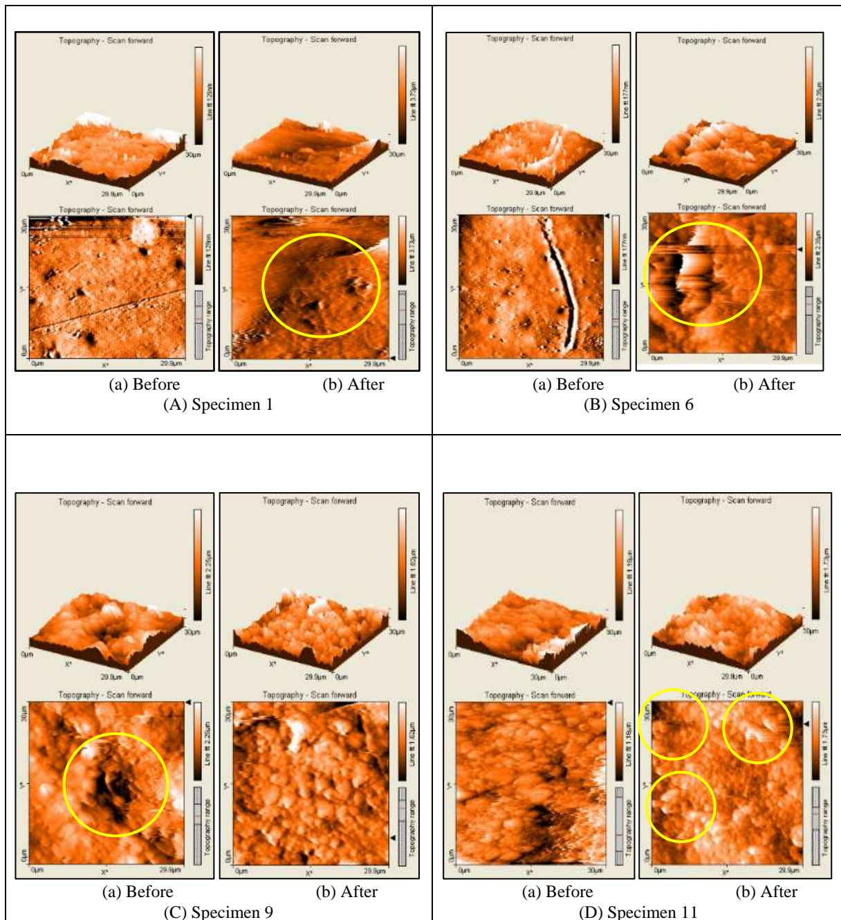
Figure 2: Three-dimensional atomic force microscopy (AFM) images illustrating the surface morphology of nanofiller composite resin specimens before and after immersion in different mouthwash solutions: (A) Syzygium cumini (Jamblang) fruit juice mouthwash, (B) 0.2% chlorhexidine mouthwash, (C) commercial herbal mouthwash, and (D) distilled water. The left column (a) displays the surface topography prior to immersion, while the right column (b) presents the post-immersion condition. Yellow circles denote regions with increased or decreased surface roughness. Scale bars are located on the right side of each image. Surface irregularities are visually represented by darker areas, which correspond to deeper or rougher surface features.
