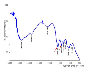
Figure 1: FTIR spectra of NaCMC produced from durian rind cellulose
