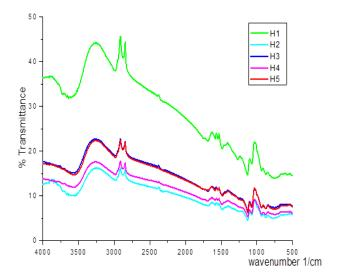
**Figure 5:** FTIR spectra of carboxymethyl cellulose-based hydrogel with variation in concentration of glycerol (H1-H5)
