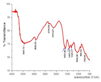
Figure 2: FTIR spectra of commercial NaCMC
