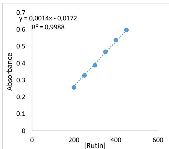
**Figure 4:** Rutin calibration curve
