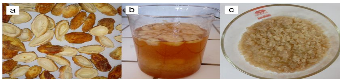
Figure 1: Extraction of polysaccharides from B. aegyptiaca Del. fruits (a) B. aegyptiaca Del. fruits, (b) alcoholic precipitation, (c) aspect of the crude extract before drying.
