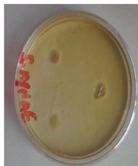
Figure 10g: Zone of inhibition at 1 mg/mL for ZnO-NPs against S. typhi
