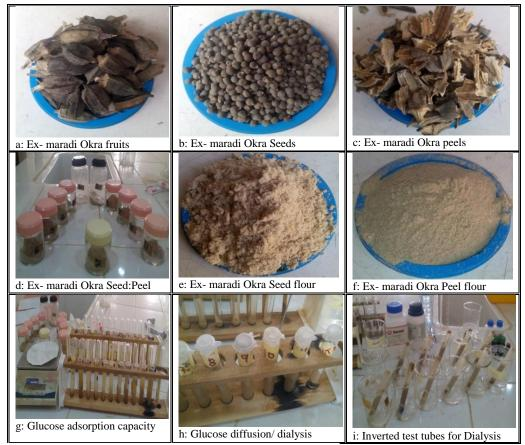
Figure 1a-i: Various components of the experimental set-ups.
