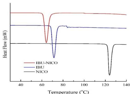
**Figure 4:** DSC thermograms of pure ibuprofen (IBU) and ibuprofen-nicotinamide cocrystals (IBU-NICO)
