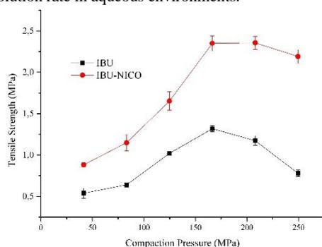
**Figure 7:** Tensile strength comparison of pure ibuprofen (IBU) and ibuprofen-nicotinamide cocrystals (IBU-NICO) under varying compaction pressures
