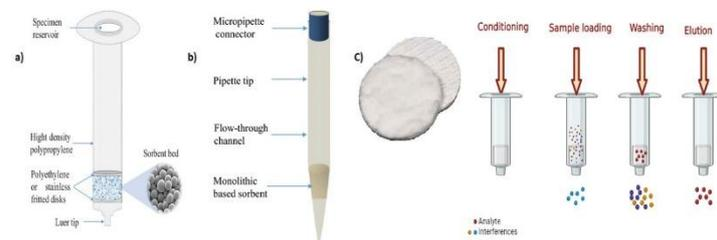
**Figure 4:** Illustration of SPE principle and common types of SPE.
