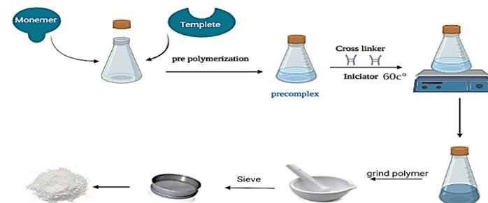
**Figure 7:** Schematic illustration of the preparation of MIP by bulk polymerization.
