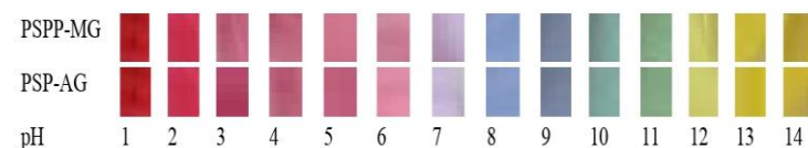
Figure 1: Colour change of (a) PSPP-MG and (b) PSPP-AG in solutions of pH 1-14
