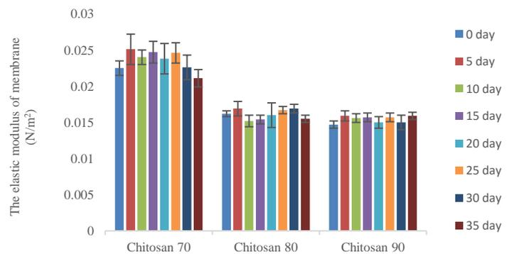
**Figure 4:** Elastic modulus of chitosan films over 35 days period
