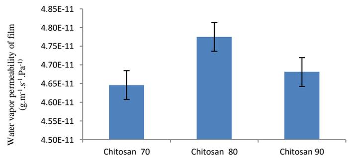
Figure 1: Water vapour permeability of chitosan films
