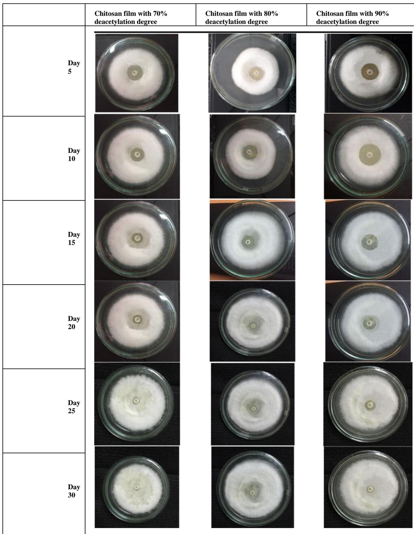
**Figure 5:** Petri dishes showing the antifungal inhibition zones of chitosan films against *Colletotrichum gloeosporioides*
