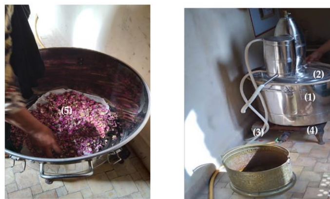
Figure 3: Hydrodistillation apparatus utilized by cooperatives in the Fes-Meknes region. The process involves placing plant material (5) within the alembic pot (1) containing water, followed by hermetic sealing with a tight lid (2). Upon heating (4), steam is generated, which effectively carries the aromatic constituents from the plant material. These constituents are then condensed within the condenser (3), resulting in the collection of hydrosols.
