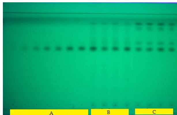
Figure 1: Results of piperine qualitative analysis using the TLC method. Piperine standart (A), BPE (B), JLPE (C).
