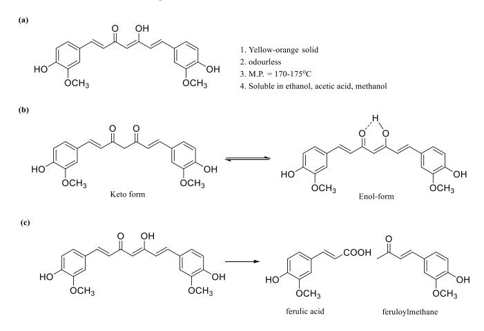
Figure 1: (a) Structure of Curcumin and its properties (b) keto-enol tautomerism and its stabilization by hydrogen bond (c) degradation of Curcumin into ferulic acid and feruloylmethane
