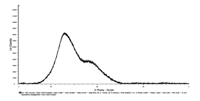
Figure 3: X-Ray Diffractogram (XPRD) graph of extracted Anacardium occidentale gum
