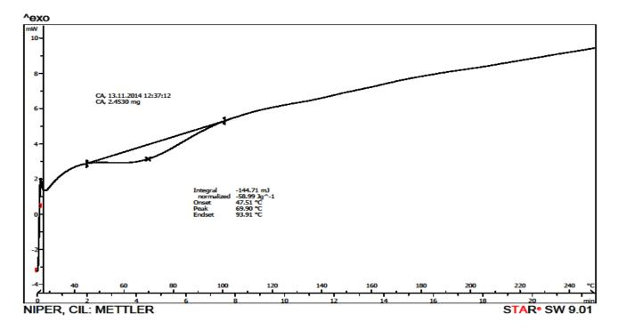
**Figure 2:** Differential Scanning Calorimetry (DSC) Thermogram of extracted *Anacardium occidentale* gum recorded in a dynamic nitrogen atmosphere (50 mL min-1), and at a heating rate of 2 °C min<sup>-1</sup>.
