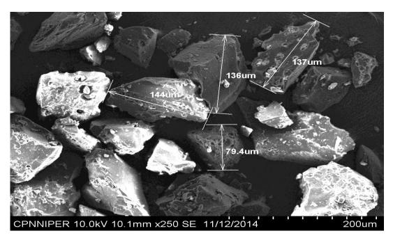
Figure 4: Scanning Electron Micrograph of extracted Anacardium occidentale gum @ x250 magnification
