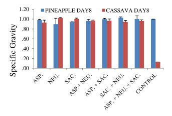
**Figure 6:** Bioethanol specific gravities of pineapple and cassava substrates using different inoculants on fermentation day 8. ASP- *Aspergillus oryzae;* NEU- *Neurospora crassa;* SAC- *Saccharomyces cerevisiae.* The mean differences were considered significant at p<0.05.
