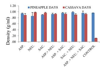
**Figure 4:** Bioethanol densities of pineapple and cassava substrates using different inoculants on fermentation day 8. ASP-*Aspergillus oryzae;* NEU- *Neurospora crassa;* SAC-*Saccharomyces cerevisiae.* The mean differences were considered significant at p < 0.05.
