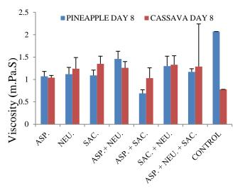
**Figure 10:** Bioethanol viscosities of pineapple and cassava substrates using different inoculants on fermentation day 8. ASP-*Aspergillus oryzae;* NEU-*Neurospora crassa;* SAC-*Saccharomyces cerevisiae.* The mean differences were considered significant at p < 0.05.
