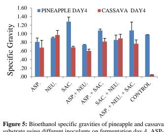
**Figure 5:** Bioethanol specific gravities of pineapple and cassava substrate using different inoculants on fermentation day 4. ASP-*Aspergillus oryzae;* NEU-*Neurospora crassa;* SAC-*Saccharomyces cerevisiae.* The mean differences were considered significant at p < 0.05.
