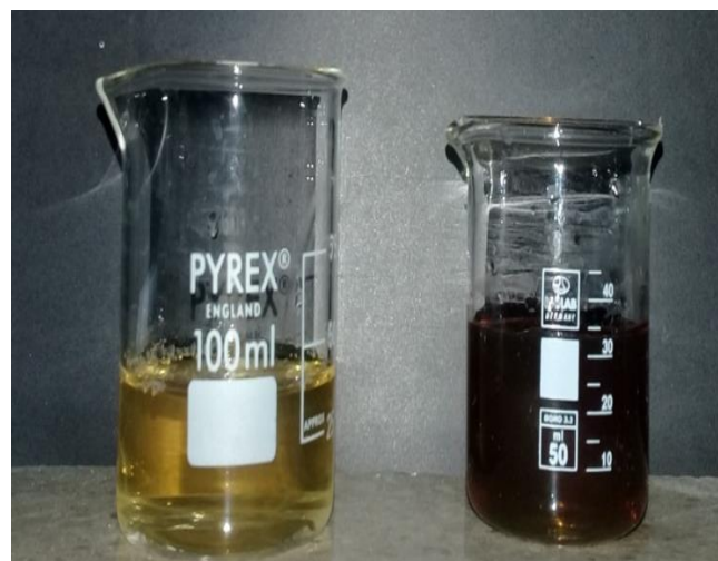
Plate 1: Colour change of the colloidal silver nanoparticle from pale yellow to dark brown as silver nanoparticles are formed.
