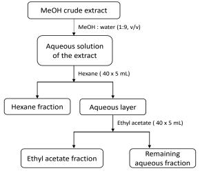
Figure 1: A scheme for fractionation of a methanolic SCG crude extract
