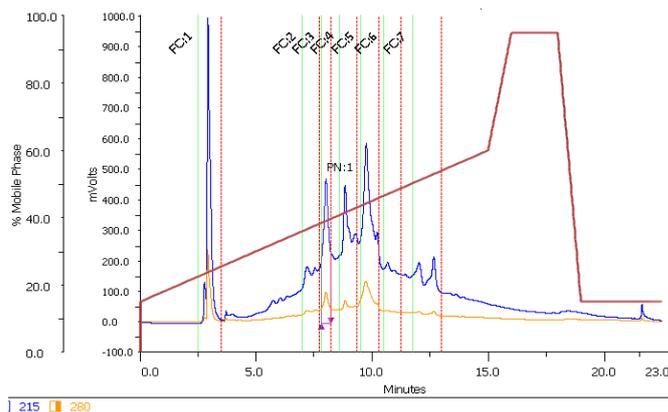
**Figure 3:** Chromatogram of preparative liquid chromatography (prep-HPLC) shows collection of seven fractions
