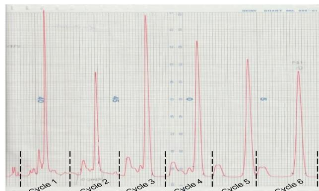
**Figure 5:** Chromatogram from recycling HPLC shows cycles of chromatographic run
