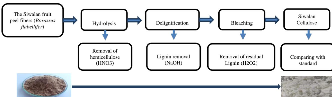
**Figure 1:** Schematic of the Isolation and Characterization of Cellulose from Siwalan (*Borassus flabellifer*) Fruit Peel Fiber
