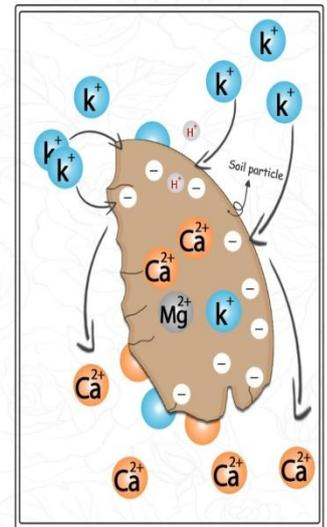
Figure 3: Ion Exchange theory
