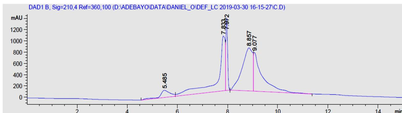
**Figure 4:** The chromatogram of Sample C was recorded at 210 nm and a flow rate of 0.25 mL/min. The chromatogram is offset for clarity. No peak for acrylamide was recorded.
