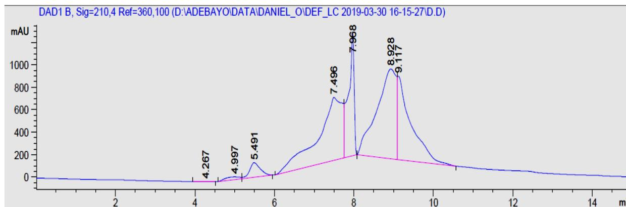
**Figure 5:** The chromatogram of Sample D was recorded at 210 nm and a flow rate of 0.25 mL/min. The chromatogram is offset for clarity. No peak for acrylamide was recorded.
