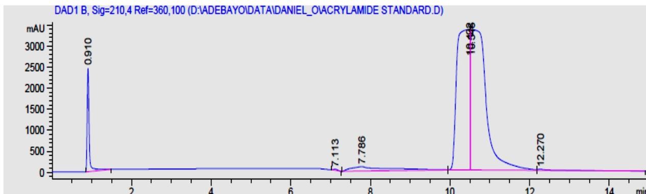
**Figure 1:** Chromatogram of acrylamide standard recorded at 210 nm and a flow rate of 0.25 mL/min. The chromatogram is offset for clarity.
