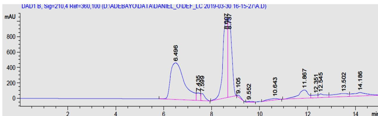
**Figure 2:** Chromatogram of Sample A recorded at 210nm and a flow rate of 0.25 mL/min. The chromatogram is offset for clarity.
