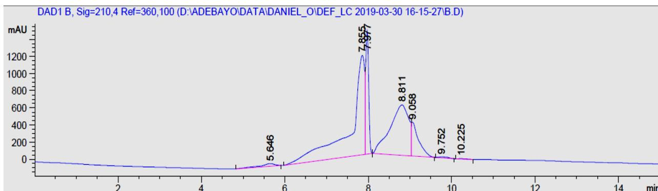
**Figure 3:** Chromatogram of Sample B recorded at 210 nm and a flow rate of 0.25 mL/min. The chromatogram is offset for clarity.
