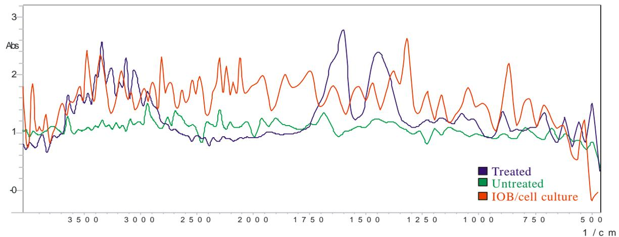
**Figure 4:** FT-IR spectrum for ammonium treated Opete bagasse incubated with crude enzyme (ENZTOB, blue), untreated Opete bagasse incubated with crude enzyme (ENZO, green), and untreated Opete bagasse incubated with inoculum /cell suspension of *Saccharomyces cerevisiae* SCPW-17 (IOB, red).
