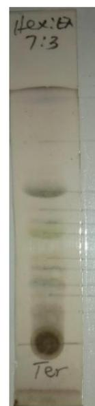
**Plate 1:** TLC chromatogram of terpenoid-rich fraction
