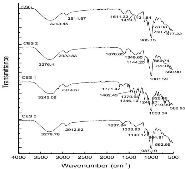
**Figure 1:** Stacked FTIR spectra of native starch (CES0), modified starches (CES1 and CES2) and sodium starch glycolate (SSG).
