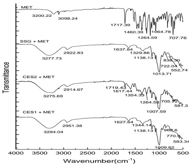
**Figure 2:** Stacked FTIR spectra for compatibility studies of metronidazole with modified starch samples (CES1 and CES) and sodium starch glycolate.
