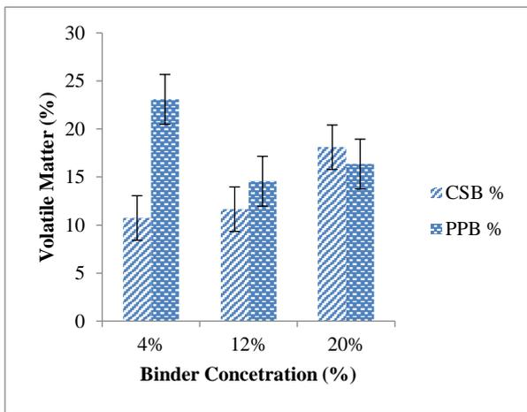
**Figure 2:** Effect of binder type on volatile matter of fuel briquette.
