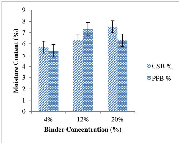
**Figure 1:** Effect of binder type on moisture content of fuel briquette.
