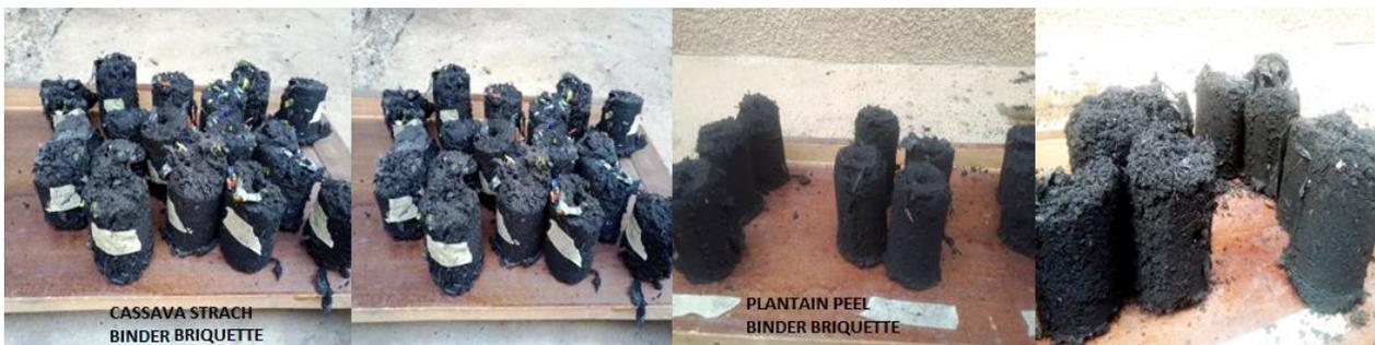
Plate I: Produced fuel briquettes from biomass waste
