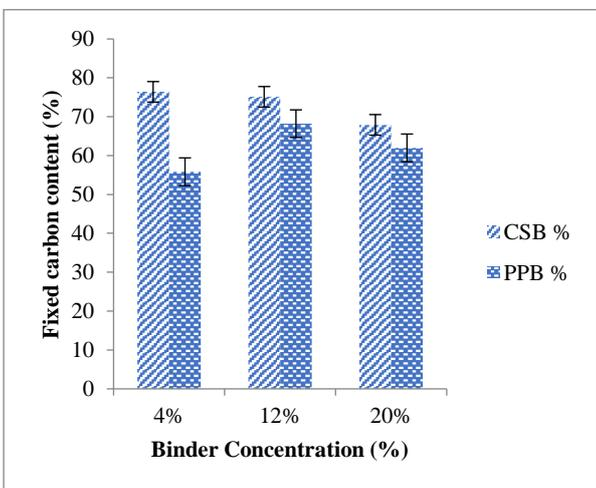
**Figure 3:** Effect of binder type on fixed carbon content of fuel briquette.
