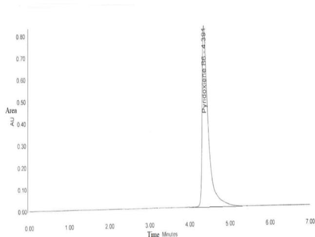
**Figure 3:** Chromatogram for Standard Pyridoxine Hydrochloride 497  $\mu$ g/mL at 280 nm
